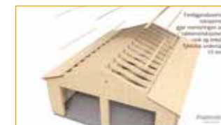
Montér undertak / rupanel
